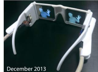
Over the last 12 months we have made a number of prototypes. Our most recent has a 3D printed frame and transparent OLED displays.
