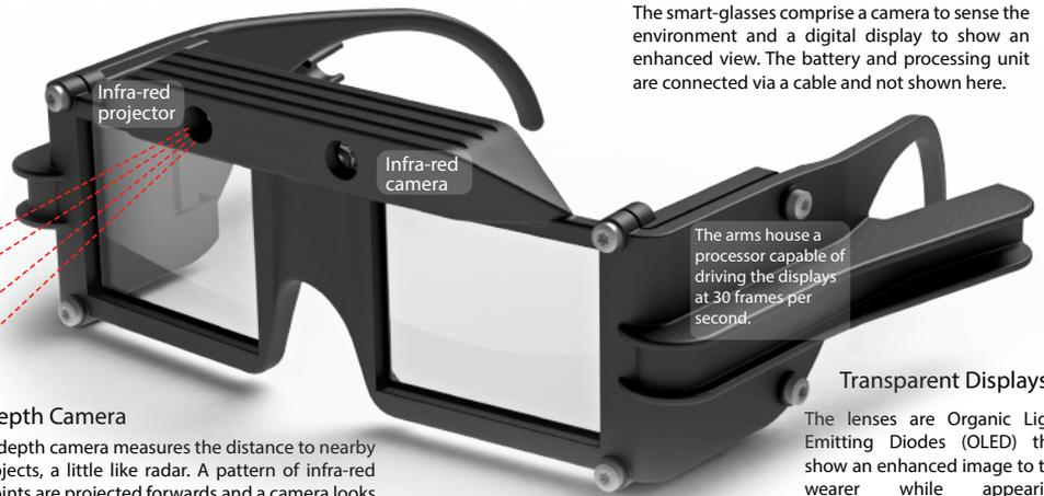
The smart-glasses comprise a camera to sense the environment and a digital display to show an enhanced view. The battery and processing unit are connected via a cable and not shown here.
